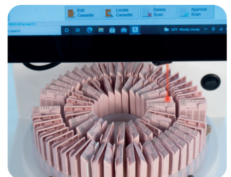
A laser pointer locates the cassettes with missing or unreadable codes
