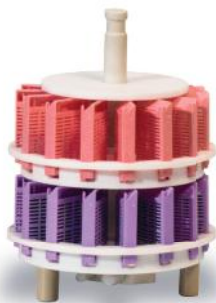
Standard - 30 cassettes For specimens 30x25x5 mm
